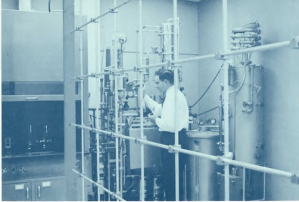
Dr. Boris Cahan adjusts multi-stage still used at Philco Research in production of hyper-pure water.
