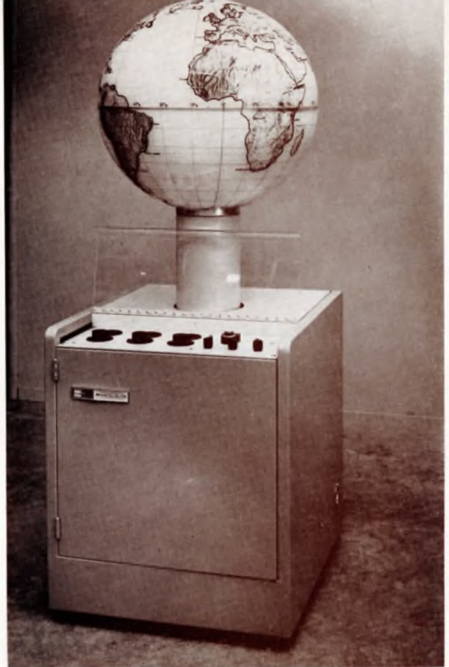
The Philco WDL Satellite Orbit Simulator can reproduce any satellite's path on the illuminated globe of the earth.
