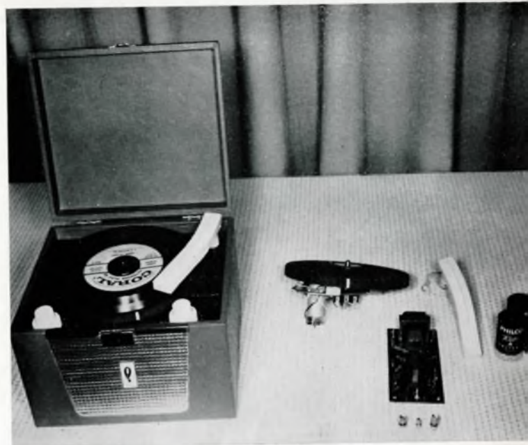
FIRST TRANSISTORIZED PHONOGRAPH developed by Philco, together with its components, emphasizes the simplicity and small size of the instrument. The "transistor" phonograph operates on four flashlight batteries without "plug-in" current. It will play 3,000 records without battery change. Three tiny transistors replace all vacuum tubes.
