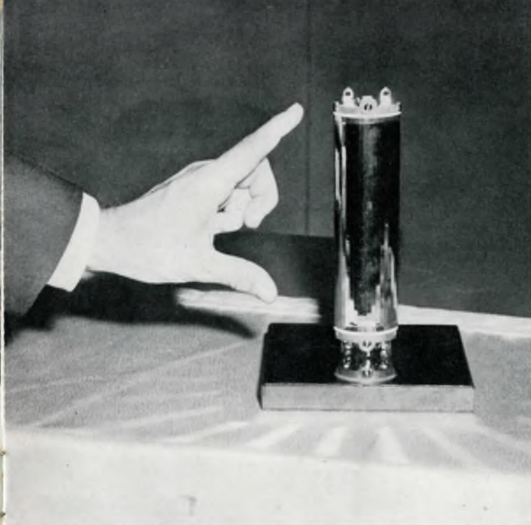
SMALL BUT RANGY is Philco's new "electrostatic" phonograph speaker. This unit, a mere seven inches high, reproduces sound uniformly up to frequencies of 20,000 cycles with virtually zero distortion. It marks a radical change from conventional speakers due to 16 vertical units, each serving as a speaker, arranged to form a half cylinder. The electrostatic speaker is used on five new Philco high-fidelity phonographs: one table model and four consoles.
