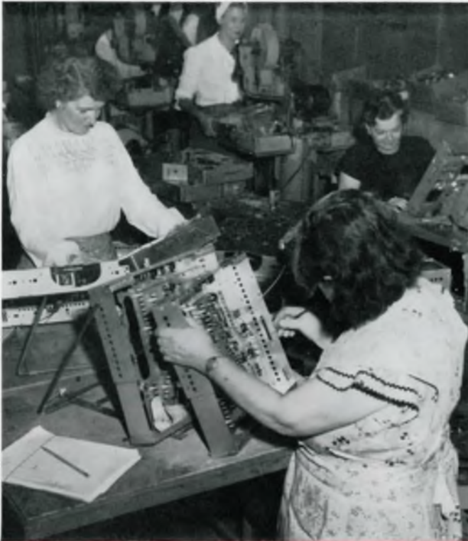
EVERY OPERATION is inspected to maintain Philco's high quality standards. Here the riveted sub-base gets a thorough examination before it is sent to the chassis wiring line.
