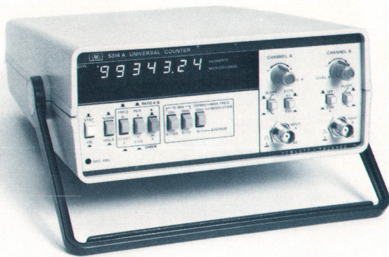
Fig. 1. Model 5314A is a low-cost two-channel 100-MHz universal counter that measures frequency, period average, time interval and ratio.
