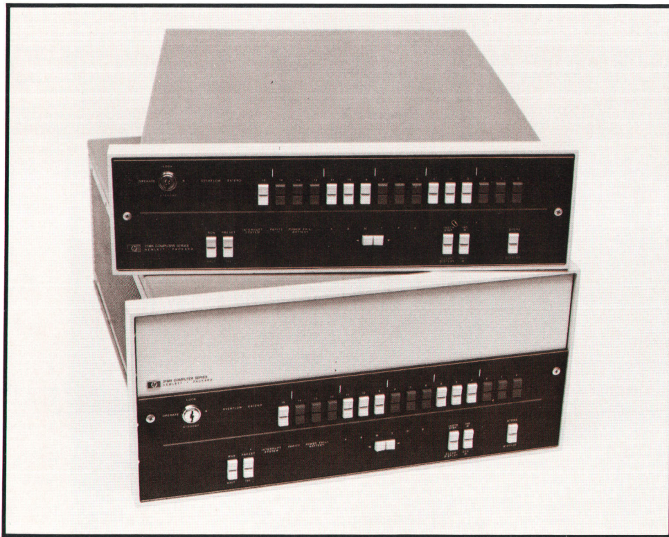
Fig. 1. The 21MX Series now consists of two computers—M/10 and M/20—with different levels of capability. Both are user-micro-programmable and have semiconductor main memory.
