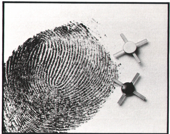
Fig. 9. Completed diode quad can be installed in circuits by conventional soldering techniques.
