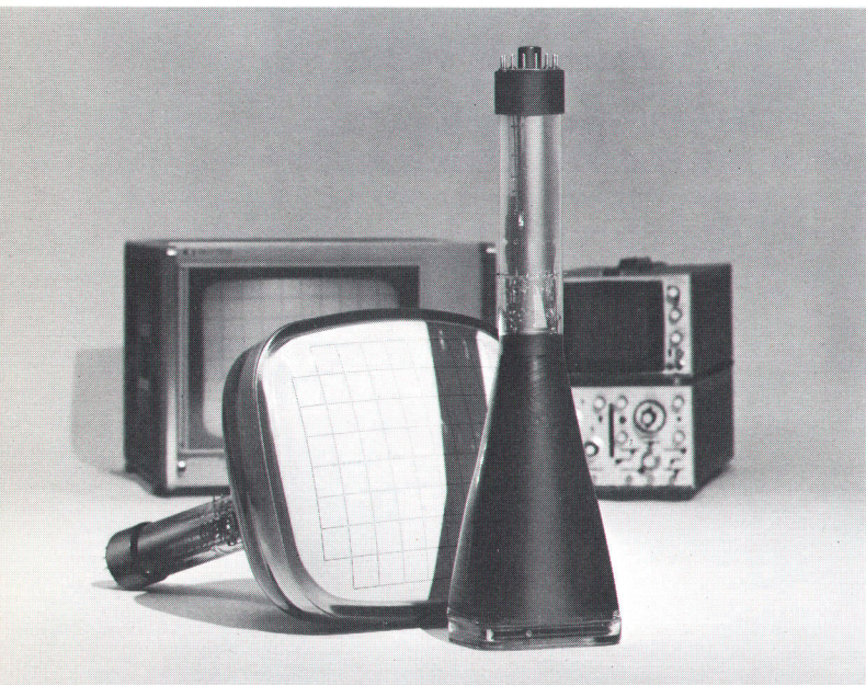
A very large CRT display in a relatively short envelope (Model 1300A CRT, left) can be obtained by suitable design of the expansion mesh. Other engineering factors appropriate to specific applications may dictate an expansion mesh design to accommodate smaller displays.
