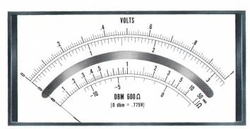
Fig. 3. Each mirror-backed meter scale for new Multi-function Meter is individually calibrated on -hp-'s servo-controlled meter calibrator. Meter face, shown here three-fourths actual size, also includes dB scale calibrated for 600-ohm systems. Meter has temperature-compensated, 100-μA, taut-band movement.
