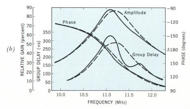
Fig. 4. Typical amplifier gain, phase, and group delay measurements, made with Vector Voltmeter in setup shown in (a). Solid curves of (b) were taken with switch on second amplifier stage open, so that second-stage gain was greater than one. Dashed curves of (b) were measured with switch closed, second-stage gain = 0. Difference
