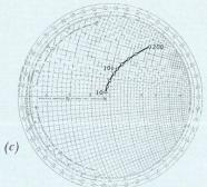
Expanded Smith chart plot of reflection coefficient of 50-ohm  $\pm 1\%$  metal film resistor attached to BNC connector. Circuit was (a) with probe B in position B1, resistor as device X, and only one directional coupler.
