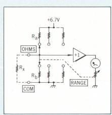
Fig. 8. Ohmmeter circuits.
