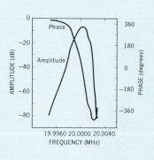
Gain and phase shift of *-hp-* Model 8442A 20-MHz Crystal Filter as measured with new RF Vector Voltmeter.
