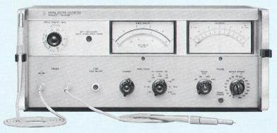
Fig. 1. –hp– Model 8405A Vector Voltmeter measures amplitudes and phase simultaneously. Instrument has frequency range of 1 MHz to 1 GHz, sensitivity of 100 µV full-scale, dynamic range of 95 dB, phase resolution of 0.1°, and is simple to operate. Thus it makes feasible many measurements which formerly were difficult or impossible.
