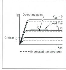
Fig. 4. Typical characteristic curves for field-effect transistor. Increase in temperature changes V<sub>gsv</sub> of load line to compensate for temperatureinduced changes of operating points in associated bi-polar transistors.
