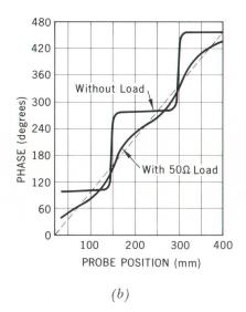
Fig. 3. Demonstration of phase-measuring capabilities of Vector Voltmeter. Phasemeter readings vs. slotted-line probe positions for setup of (a) are plotted in (b). Steepest portion of (b) curves is shown expanded in (c). Maximum rate of change of phase of 50°/mm, or 2° per human hair diameter, is easily measured. With slotted line terminated in 50 ohms, maximum deviation of phase from linear, theoretically 22.8° for measured VSWR of 2.26, is measured as 22°. Frequency is 1.003 GHz.
