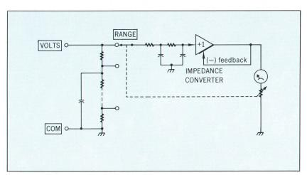
Fig. 6. Block diagram of new multi-function meter in dc voltage measuring configuration. Range switch at input attenuator also adjusts sensitivity of meter circuit.
