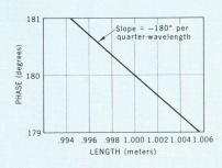
Phase versus length of cable for system shown in block diagram, calibrated at 75 MHz (quarter-wavelength = 1 m). Phase resolution of VVM is 0.1°, allowing length to be determined within 0.6 mm at 75 MHz, or more accurately at higher frequencies.
