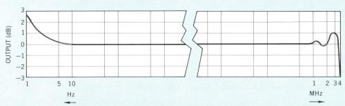
Fig. 1. Frequency response of new -hp- Model 427A Multi-function Meter is essentially flat from 10 Hz to 1 MHz but useful response extends to 4 MHz at 3-dB point.
