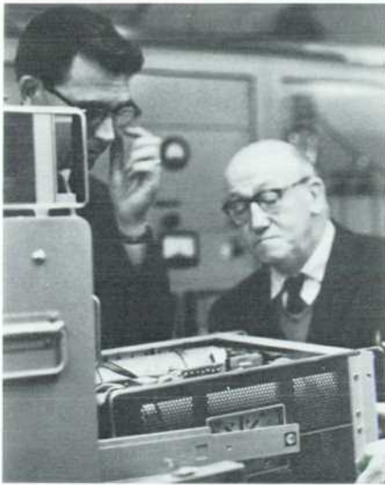
Fig. 10. Dr. L. Essen, who developed world's first Cesium 133 atomic-controlled frequency standard at National Physical Laboratories, examines compact cesium-beam frequency standard that controls traveling clock.
