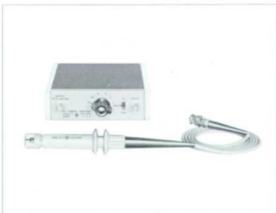
Fig. 2. -hp- Model 1110A AC Current Probe and Model 1111A Amplifier. Probe clips around conductor being measured.
