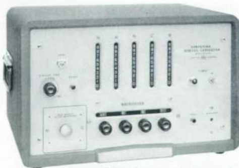
Fig. 1. Gate time in new -dy- 2500 Counter is adjustable in 0.1 millisecond steps from 0.1 millisecond to 0.9999 second to enable measurements to be made directly in any desired unit such as rpm or gallons/hour.
