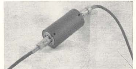
Transistor Preamplifier can be mounted directly at the microphone to give increased gain and lower the noise level on long microphone runs.
