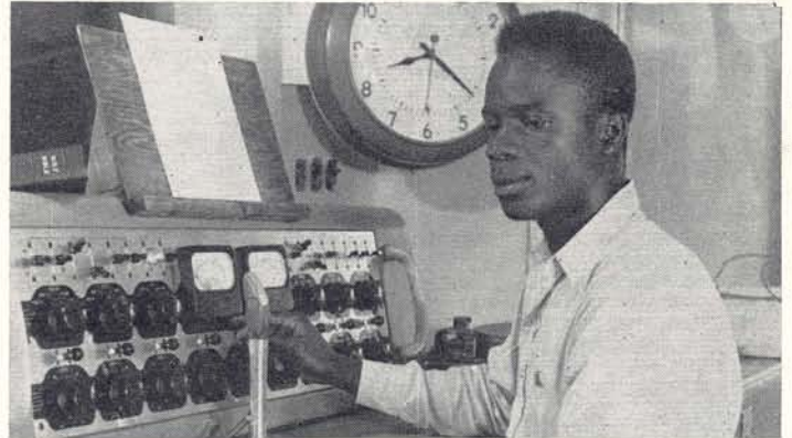
Gates SA-50 dual channel control console provides the flexibility required in a multi-lingual operation.
