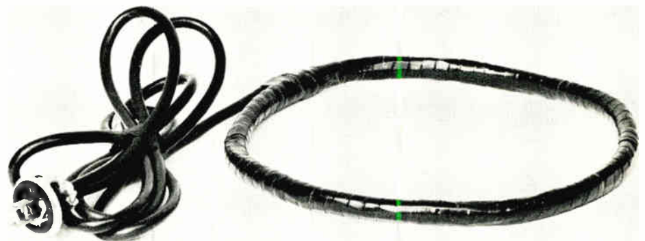
Fig. 2. Degaussing coil constructed as described.
