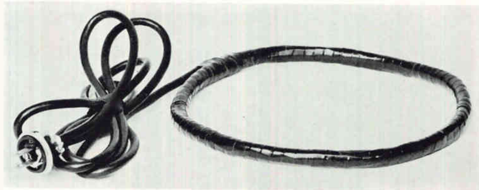
Fig. 2. Degaussing coil constructed as described.
