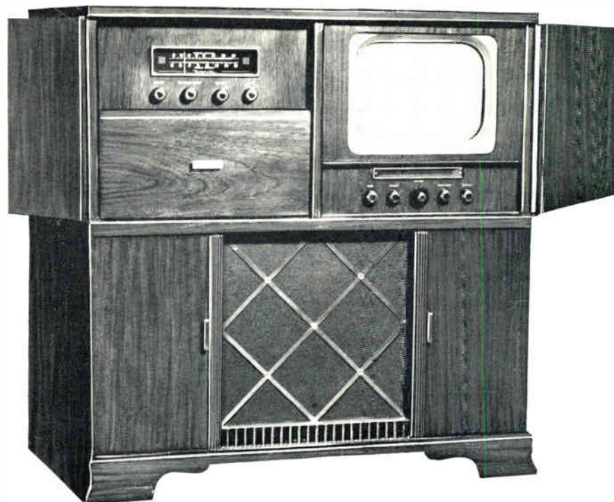
Fig. 5. Motorola Model VF-102 FM-AM phonograph combination after it was converted to use a General Electric 14CP4 picture tube.
