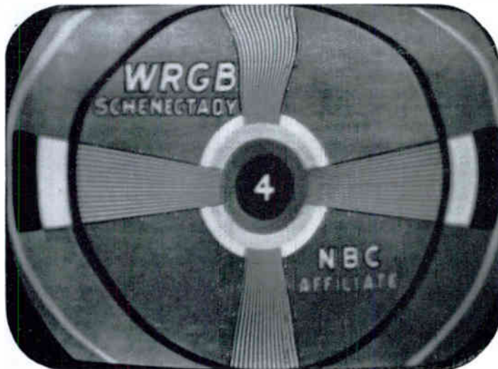
Tele-Clue No. E-59 —The curve and waviness which appears only at the top of the picture may be due in the General Electric Model 810 line of receivers to the resistance of R98 in Fig. 1 being too low. When replacing use a 56000-ohm resistor.
