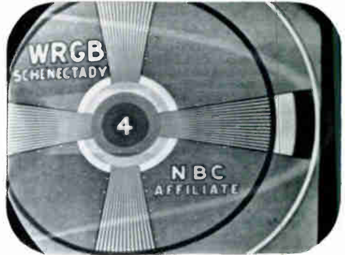
Fig. 2. Horizontal fold-over usually caused by the horizontal retrace being too slow.
