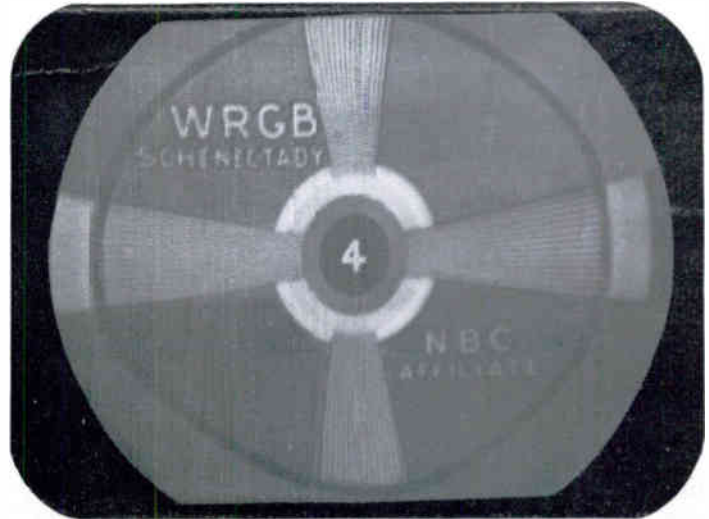
Tele-Clue No. H-60 —A washed out picture may be due to a low emission or "soft" picture tube. This same type picture will result when the voltage on the No. 2 grid of the picture tube is reduced by leakage to ground.
