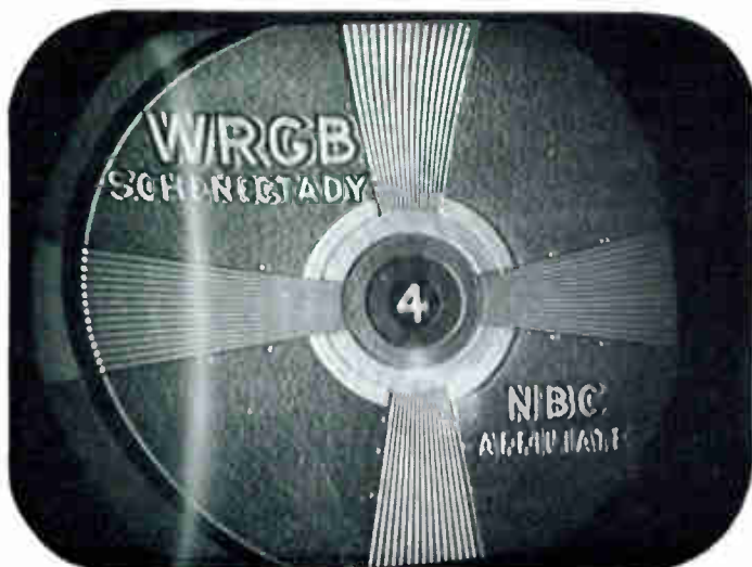
Fig. 1. The faint vertical white line at the left may be due to a defect in the damping circuit. The fine tuning control was adjusted to accentuate the whites.
