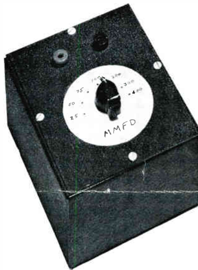
Fig. 1. Photograph showing the completed capacitor substitution boxes.
