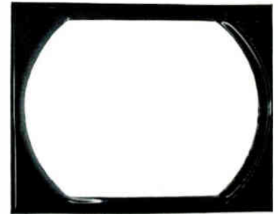
Figure 4. Twenty-four inch plastic mask used to replace viewing screen on General Electric Model 910 receiver.
