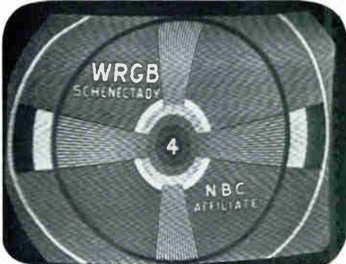
Tele-Clue No. J-72—This type of interference known as oscillator radiation is due to the oscillator in some nearby receiver acting like a miniature transmitter and radiating a signal. This signal is picked up by the antenna or lead-in together with the desired signal and amplified resulting in the interference pattern shown above.
