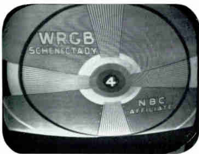
Tele-Clue No. D-69—Leakage across C308 in Fig. 13 of one megohm resulted in the bottom being squeezed which could not be corrected by adjusting the height or vertical linearity controls. Leakage of more than one megohm could be corrected by readjustment of the height and linearity controls. Additional leakage resulted in a further reduction of the lower half.
