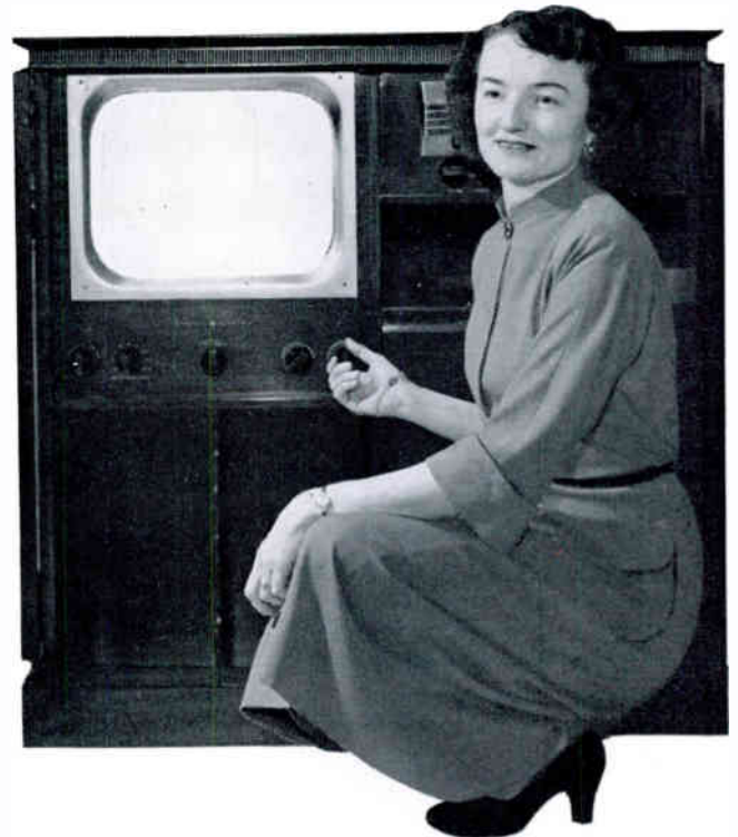
Fig. 2. General Electric Model 820 after being converted to use a 16KP4 picture tube.
