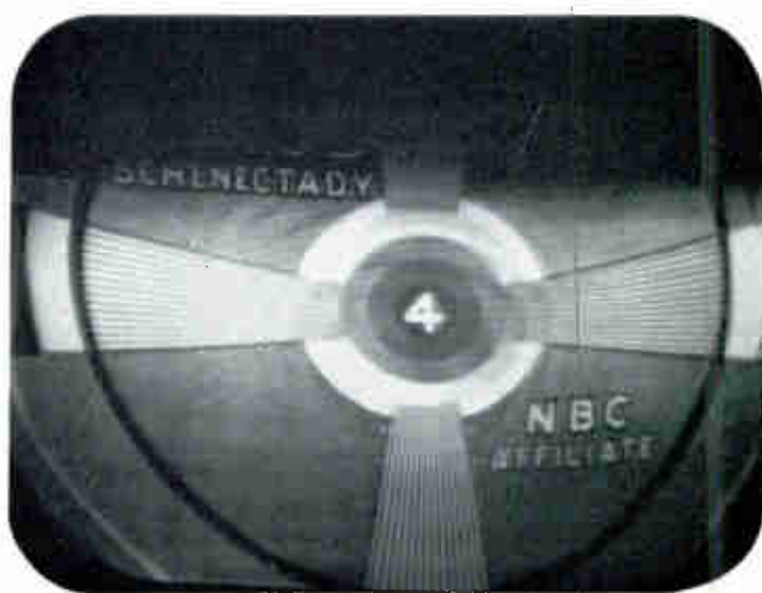
Tele-Clue No. D-70—Leakage across C311 in Fig. 12 of three megohm resulted in the top portion of the picture being darkened. As this resistance was increased the depth of the dark area decreased and as the resistance was decreased the depth of this area was increased as shown in Tele-Clue No. 71. Due to this section of V9 being part of the blanking circuit, a gassy tube will result in a reduction of screen voltage on the picture tube thereby blanking out the picture tube completely.
