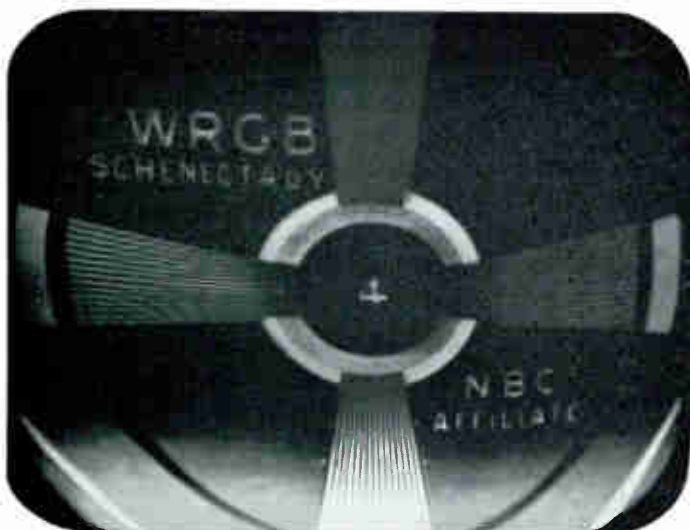
Tele-Clue No. D-71—This illustrates the result of one and one-half megohm leakage across C311. The brightness and contrast controls were advanced.
