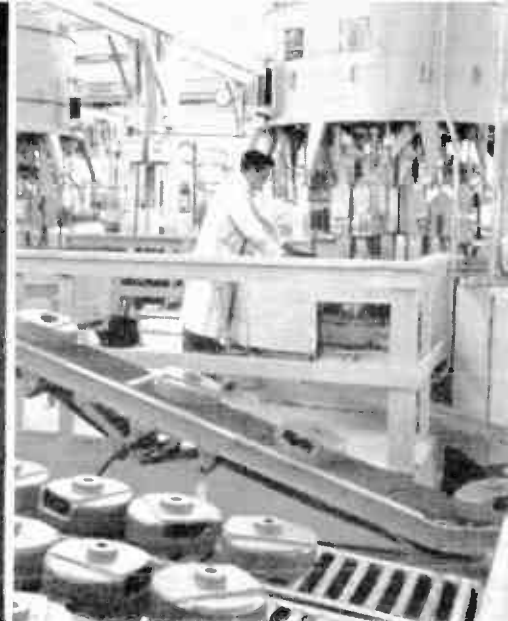
MOTOR END SHIELDS are machined and drilled by automatic machines at multiple stations, then are moved to assembly area by conveyors.
