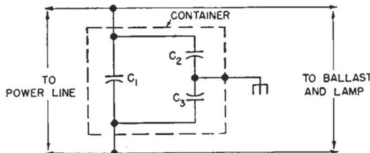
Commercially-made filters designed especially for fluorescent lamps are made by several firms. Among these, General Electric has two types that use the above circuit. One is the catalog number 25F214, designed for permanent lamp installations. The other, catalog number 25F890, is recommended for portable lamp fixtures. Your local G-E Apparatus Sales office will tell you where they can be obtained. Another type which should be available from most radio parts distributors is the Sprague IF-37.
