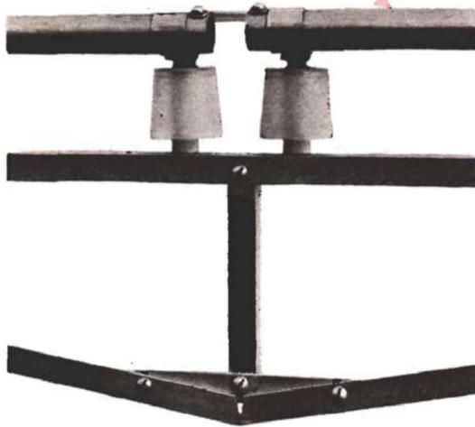
Fig. 6. Detail view at the center of the element support trusses. The element sections are spaced  $1\frac{1}{4}$  inches and the phasing line is fastened to the tubing with a spacing of 2 inches between hole centers.
