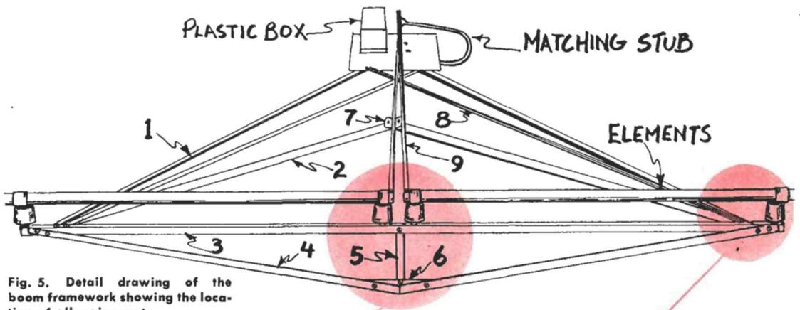
Fig. 5. Detail drawing of the boom framework showing the location of all major parts.
