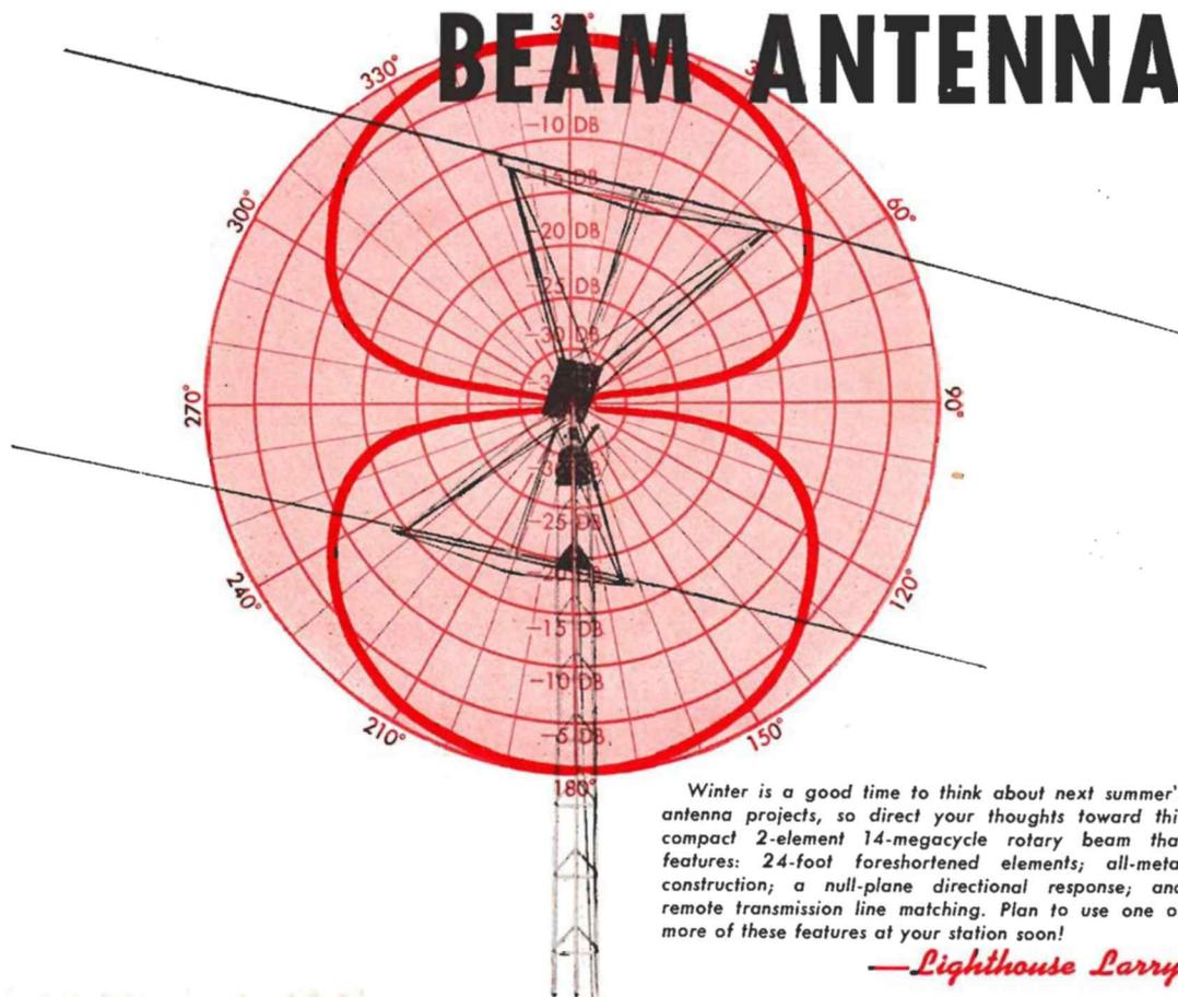
Winter is a good time to think about next summer's antenna projects, so direct your thoughts toward this compact 2-element 14-megacycle rotary beam that features: 24-foot foreshortened elements; all-metal construction; a null-plane directional response; and remote transmission line matching. Plan to use one or more of these features at your station soon!
