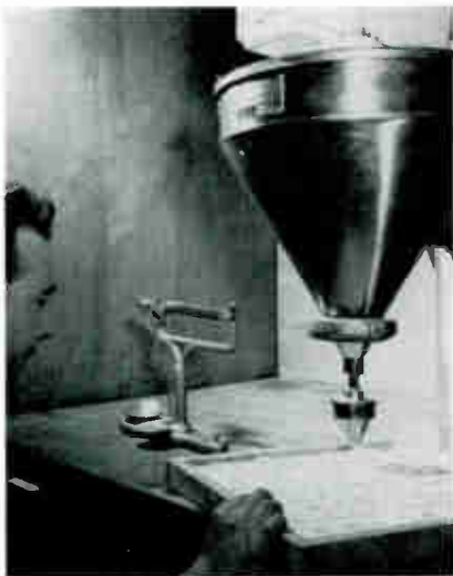
This machine, used in the medical industry to measure critical chemicals, doles out a precise quantity of phosphor material for each tube screen.
