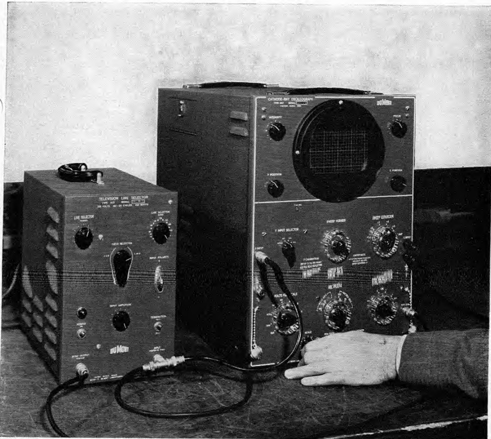
Figure 8. Type 327 with Type 325 Line Selector for television station adjustment and maintenance work.
