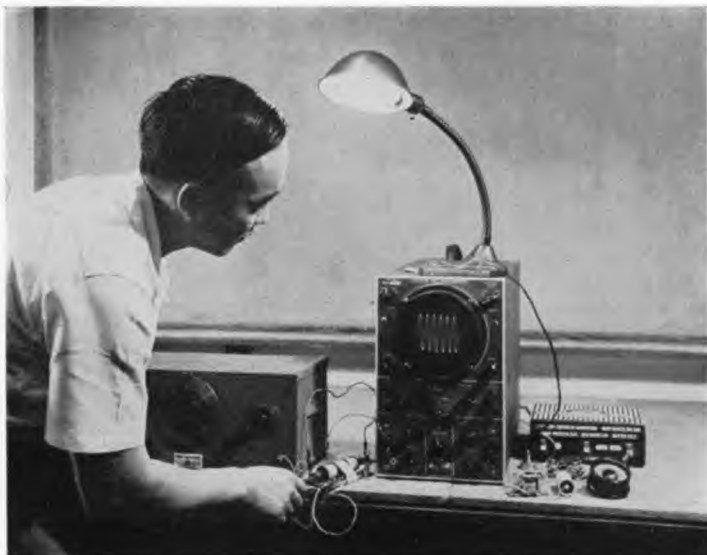
Figure 3. Unhardened drill blank being inserted into differential transformer. Result: deflection on oscillograph, light remains on
