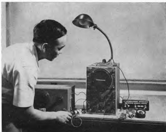
Figure 4. Hardened drill blank being inserted into differential transformer. Result: no deflection, light goes out
