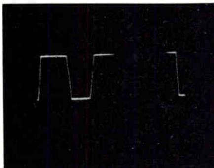
Figure 1. A portion of this oscillogram is missing because the exposure time was less than one sweep cycle
