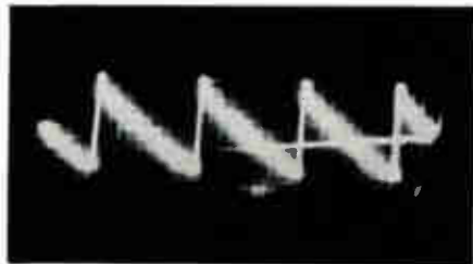
Figure 4. This oscillogram was deliberately over exposed to record the high-writing-speed portions of the trace
