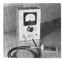
Fig. 1. Transistorized Hum Stethoscope Ready for Use. The hum probe is shown plugged into the input jack, J., See Figure 8 for identification of components.
