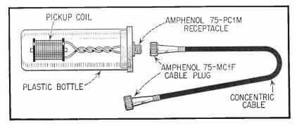
Fig. 7. Details of Hum Probe.
