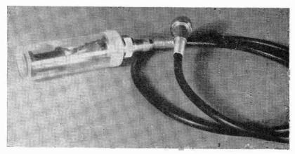
Fig. 5. Assembled Hum Probe. See Figure 7 for identification of parts.
