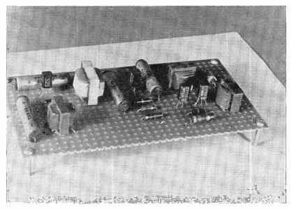
Fig. 3. Completed Circuit Board. Most of the circuit components are mounted on this  $6\frac{1}{2}$ " x  $3\frac{1}{2}$ " perforated phenolic board. See Figure 4 for identification of components.
