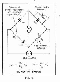
equivalent series resistance of the capacitor or inductor under test. The equivalent series resistance value subsequently is used in the computation of power factor, dissipation factor, or Q. Direct-reading bridges intended for
