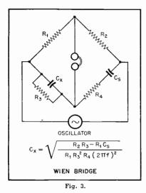
priate frequency and the detector must be a sensitive a.c. instrument, such as a v. t. voltmeter, cathode ray oscilloscope, electron-ray tube, or high-resistance headphones.
