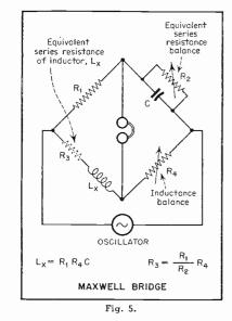
For simplicity, radio service bridges employ 60 or 120 cycles, since these frequencies are easily obtained without an oscillator.
