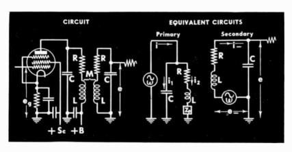
Fig. 1. Universal reference circuit and a simplified equivalent.
