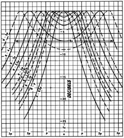
Fig. 2. Here the scale of abscissae is pure number: that is, units of p=1/Q. To convert to frequency, multiply by fo. For example, if the Q of the coils is 20, and the center-frequency is fo=10 mc, then each division (p) represents pfo cycles=0.05 x 10 mc=500 kc.
