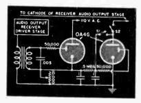
Fig. 4. An alarm system without relays.
