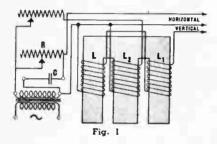
Two identical coils L and L<sub>1</sub> having a great many turns (say several thousand), are inserted on the outer legs. They should be tight-fitting. Windings from two high-resistance chokes such as the replacement components for small ac-dc receivers provide satisfactory coils here. The center leg can be a similar winding or a larger one but should fit the center leg rather tightly.
