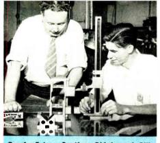
G. A. Exley, Section Chief, and Bill Britton checking dimensions on a casting with a vernier height gage.
