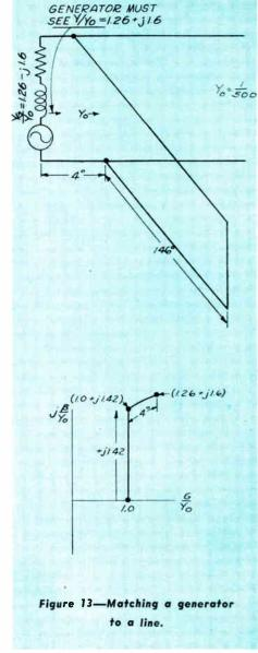
power transfer, to a line with  $Z_o = 500$  ohms. A single stub will be used. For a match, the admittance at the generator terminals must be the conjugate of the internal admittance of the generator. Per unit generator admittance is  $\frac{Y_G}{Y_o} = 1.26 - j \ 1.60$ . Hence the perunit admittance at the generator terminals must be  $1.26 + j \ 1.60$ .
