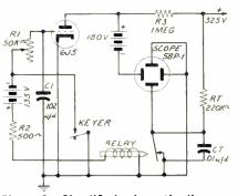
Figure 3—Simplified schematic diagram of sweep circuit No. 2.
