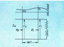
Figure 5—Standing wave of voltage on transmission line.
