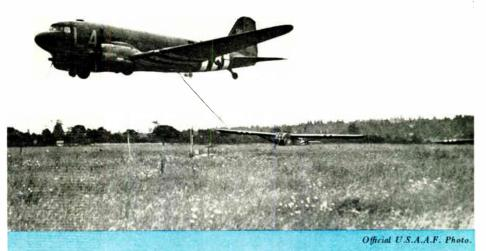
Pickup method of launching gliders has been used successfully in both theatres of war where supplies and troops have been landed or wounded men must be evacuated in areas too small for take-off of a plane with glider attached. Photograph shows a plane which participated in "D" day operations as it approaches a ground station erected on a field in France to launch a CG-4 glider.
