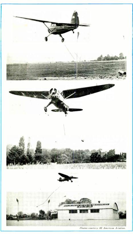
Top: Ground rope is snagged and freed from poles, and plane begins immediate pull-up to clear all obstructions.
