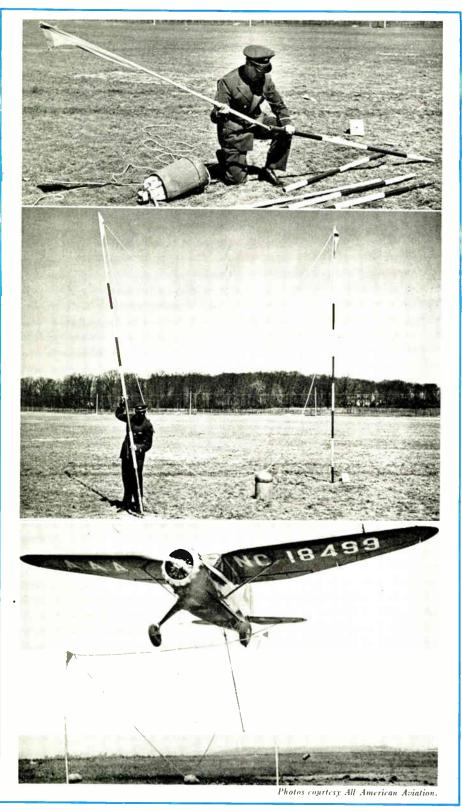
Top: Messenger assembles portable ground station equipment prior to arrival of pickup plane.
