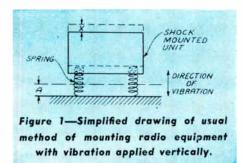
Figure 1 represents a unit mounted on equal springs, equally loaded, with vibration applied in the direction of the axis of the springs. The body moves only in the direction of the axis of the springs. To calculate the performance of this unit, proceed from the differential force-acceleration equation
