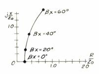
Figure 2—Per unit impedance curve for line terminated in resistance 0.2 times Zo.
