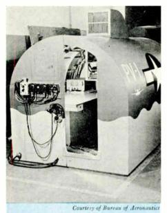
Crew training cubicle for PV-1 with MI-22A Station Box and controls at left of opening, and MN-26 Radio Compass on shelf at right of navigator's station.
