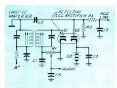
Figure 1—Conventional second detector-A. G. C. Rectifier System.
