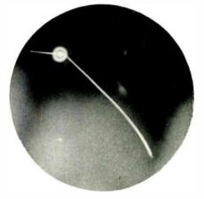
Figure 7—Horizontal sweep starting at the same time the switch contacts open.
