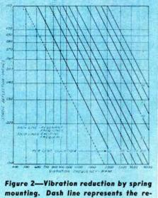
mounting. Dash line represents the relation between resonant frequency and static deflection. Solid lines represent the isolation obtainable over a range of applied frequencies for all common values of static deflection.
