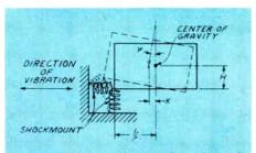
Figure 3—Schematic drawing of usual method of mounting radio equipment with vibration applied horizontally.
