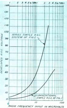
Figure 3—Comparison of A.G.C. bias voltage developed by systems of figures 1 and 2. Bias was not applied to preceding amplifier tubes when readings were made.
