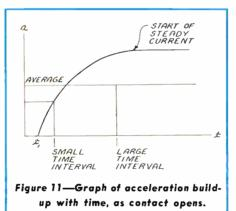
The known interval of time before the arc forms is 200 microseconds after the contacts start to open. The simplified formula gives  $s = .1038 \times 10^{-3}$  inch which value is, of course, in error on the larger side. It is apparent therefore that the formula selected should be governed by the accuracy required and the particular interval being sought.
