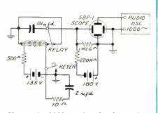
Figure 4-1000 cycle circuit used to time travel of relay armature from unenergized position to closed position.
