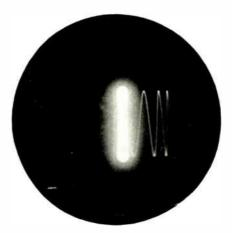
Figure 10—Pattern when 1000 cycle wave is used to time travel of switch armature from the unenergized position to the closed position.  $6J5\ tube\ starts\ to\ conduct\ and\ the\ sweep\ starts)\ in\ the\ formula$
