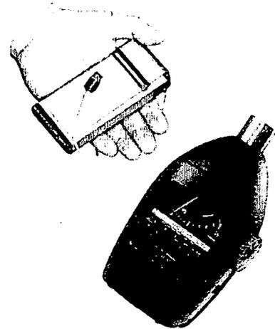
**More accurate measurements** Of the three types of sound-level meters previously allowed, only the Types 1 and 2 would be authorized under the proposed regulations — the lower-accuracy Type 3 would no longer be acceptable. Measurements must
