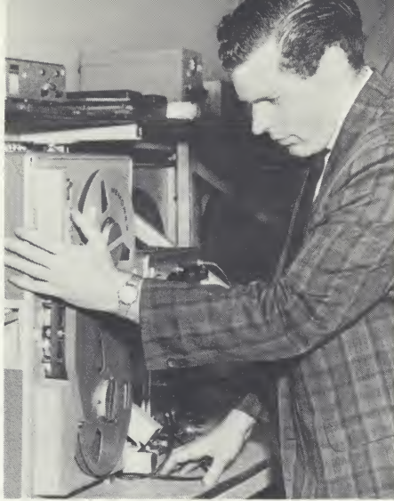
Two Ampex FR-1300 instrumentation recorders aboard high speed test train are used alternately for continuous data recording on long test runs. Over 100 different multiplexed measurements showing actual performance at high speeds are recorded on five data channels.
