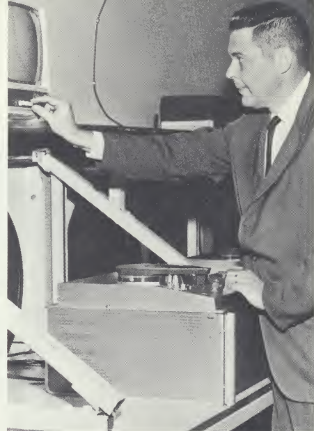
One of two Ampex VR-7000 portable videotape recorders aboard test train. Closed circuit cameras, each connected to one recorder, are located on the roof and step well to observe pantograph motion and wheel action.
