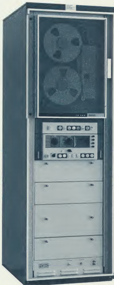
Single-channel Ampex FR-900 recorder, also used in this development.
