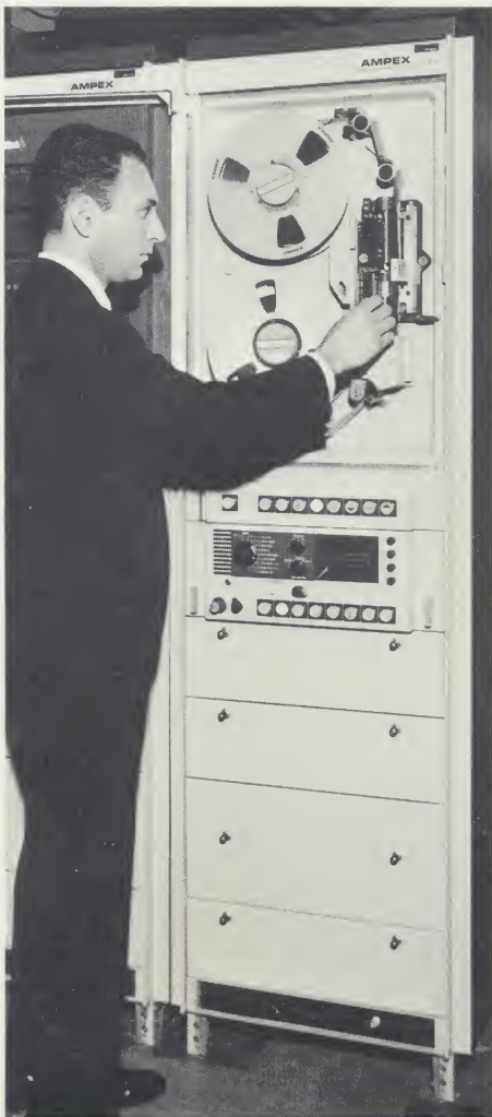
FAA project engineer adjusting the two-channel Ampex FR-950 rotary head recorder.
