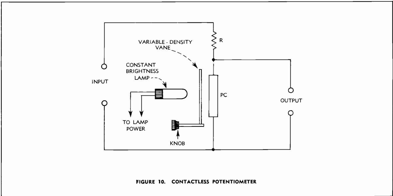
FIGURE 10. CONTACTLESS POTENTIOMETER
