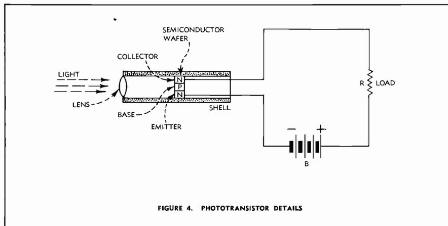
FIGURE 4. PHOTOTRANSISTOR DETAILS
