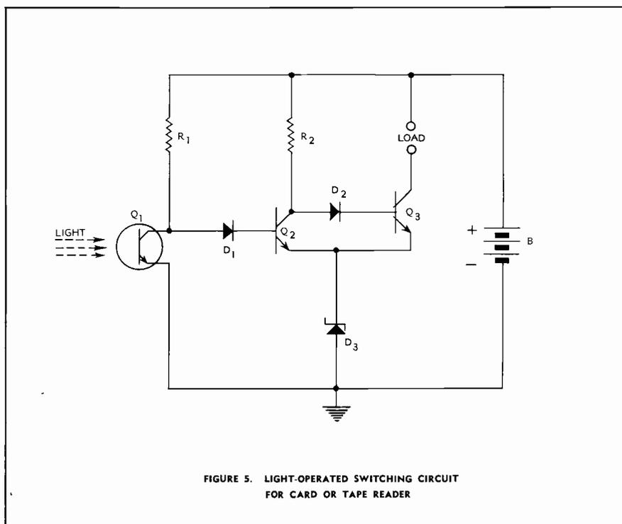
FIGURE 5. LIGHT-OPERATED SWITCHING CIRCUIT FOR CARD OR TAPE READER
