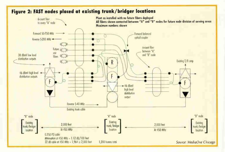
plains, resides on the existing trunk cable. The laser count typically remains the same, but output power values are increased. If further segmentation is required in the return, an additional optical transmitter may be added to the so-called "B" node locations via the six-count optical cable with limited service interruption, he says. (See Figure 3 on page 66.)
