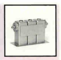
The filter achieves more than 15 dB rejection at +/-8 MHz from center frequency and more than 40 dB rejection at +/-22 MHz from center frequency. A minimum of 14 dB return loss is maintained in the passband. The filter can be tuned to any 6 MHz channel in the 470 MHz to 890 MHz range and comes in 50-ohm or 75-ohm configurations.
