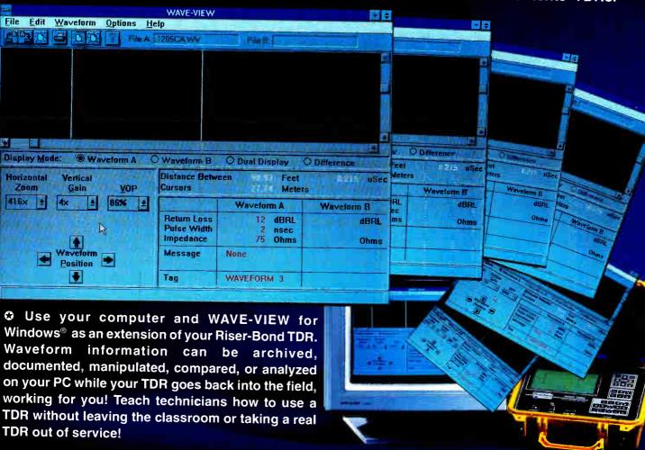
Unlike any other TDR's software program, WAVE-VIEW not only allows you to recall stored waveforms on your PC, but it also displays the TDR's function keys. You can actually increase the vertical gain, zoom in and out, manipulate the waveform, adjust the cursors, and change VOP, right on your computer!
