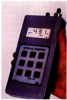
(850, 1,310 and 1,550 nm) are available with 0.1 dBm resolution. Dynamic range is +5 to -60 dBm at 1,310/1,550 nm and +5 to -55 dBm at 850 nm (+3 dB). Laser sources are available in 1,310 and 1,550 nm wavelengths. LED sources are available for 850 or 1,300 nm wavelengths.
