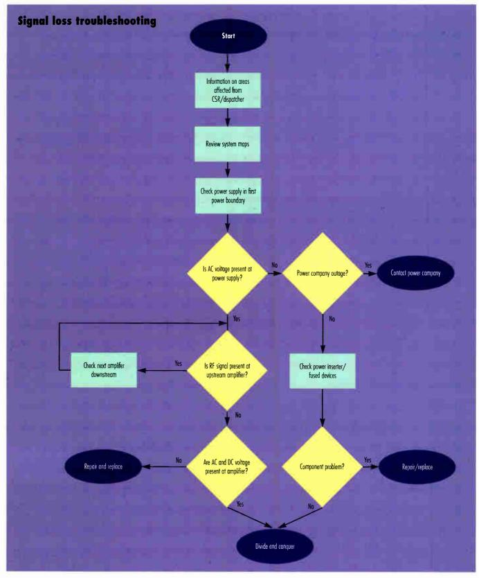
pinpoint a fault. A span of cable containing a short also can be identified by measuring amperage draw with a VOM. Apply the divide and conquer method to again save time and energy. Once the span has been identified, the TDR and/or leak detector
