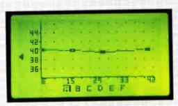
When equipped with the Multiplexer Option, the 9580SST accepts signals from up to 8 separate test points and analyzes sweep & ingress from each individually, returning data to as many as 6 SSR field units (A thru F) connected to it.
