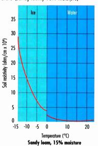
In some places, ensuring low resistivity is as simple as driving a ground rod into a subsurface soil layer that has a relatively permanent and conductive moisture content. In the absence of such favorable conditions, though, there are other options for improving soil conductivity. These include filling the ground rod hole with bentonite, treating the soil with a salt (such as copper or magnesium sulfate, or rock salt), or using a ground enhancement material.
