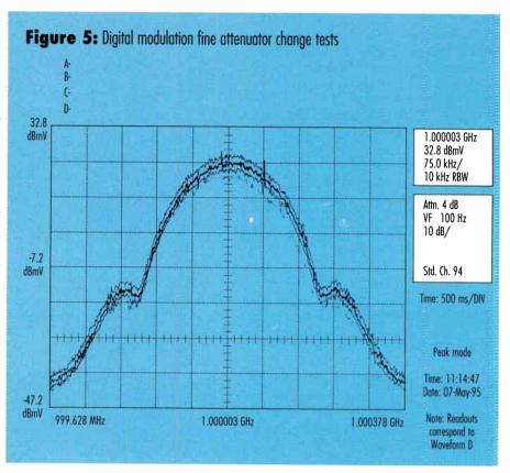
cally 54 dBmV. When all the calculations and performance measures are taken into account, we find that the dynamic range for both analog and digital, or mixed hybrid, signals is about 60 to 70 dB, depending on the number of carriers involved. This can lead to marginal results, which may require the use of an external input preselector to reduce the input signal loading.
