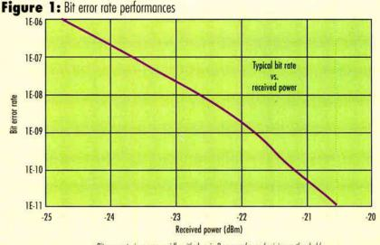
Bit error rate increases rapidly with drop in Rx power beyond minimum threshold.
