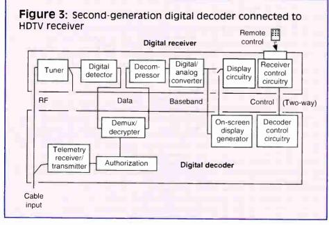
Both MPEG-2 and DigiCipher work by: a) removing redundant picture elements; b) motion prediction; and c) very efficient code generating algorithms. While digitized, uncompressed NTSC TV requires a data rate of about 100 Mb/s, acceptable quality encoded pictures have been reduced to 3-6 Mb/s.
