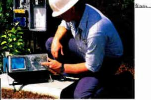
(ABOVE) THE 2714 CABLE TV SPECTRUM ANALYZER AUTOMATES ALL COMMON CABLE SYSTEM SPECTRAI. MEASUREMENTS, INCLUDING THE FCC RF PROOF-OF-PERFORMANCE REQUIREMENTS.
