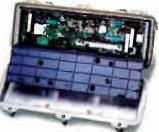
**FUTURE READY** - 1.5 GHz platform for bandwidth expansion, reversible module, and a replaceable lid for flexibility.
