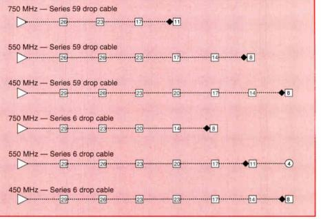
cies. Using Series 11 cable for drops at 750 MHz will closely resemble minimum tap port levels at 450 MHz using Series 6 drop cable. Since the most common drop cable found in systems today is Series 6 or 59, the accompanying figure will reference these two types of cable in the design comparison.
