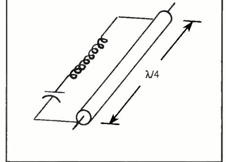
an inductor, and the open-circuited coax will take on the characteristics of a capacitor.
