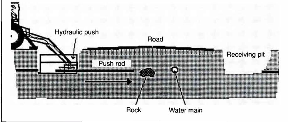
the optical cable is pulled through the duct for added protection of the cable. The metal pipes generally extend through the pit dug on each side of the road to protect the cable from added stress when the earth settles.
