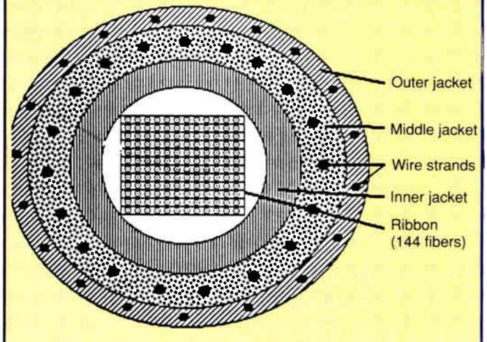
low Kevlar material that provides added tensile strength. Kevlar is the material bulletproof vests are made from. It is usually considered to be a load-bearing member of the cable. It is also non-conducting and therefore is ideal for dielectric cables.
