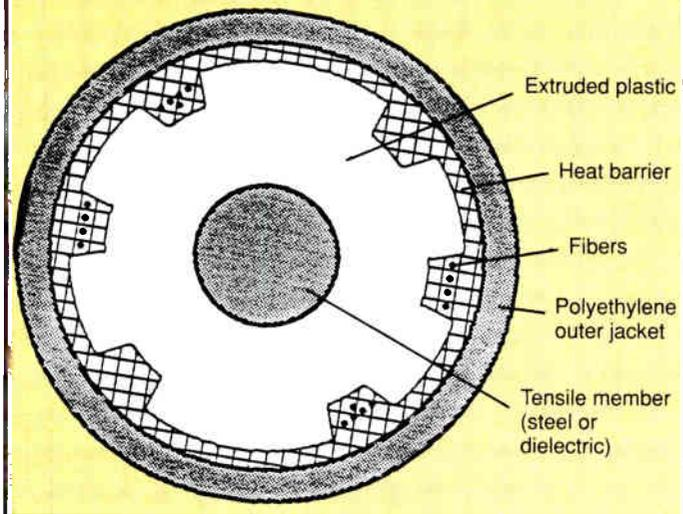
**Figure 4:** Ribbon cable design
