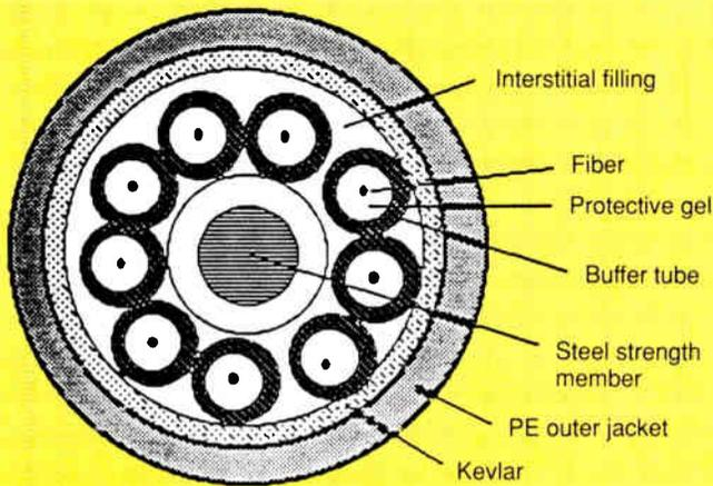
**Figure 2:** Buffer tube allows safe cable stretching
