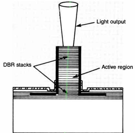
tration of light intensity at the laser's emitting facet will increase laser life and reduce risk of damage to the facet. Having lasers made with vertical emission will enable testing of the laser properties while on the wafer, in contrast to conventional lasers where each one must be mounted and tested individually. The yield of the mounting operation will increase dramatically.
