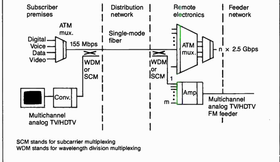
four analog FM video channels (out of a total of 61 channels offered) and two digital voice channels. Both voice and video services are subcarrier-multiplexed in a 200 MHz signal. The voice capabilities include both standard POTS and narrowband ISDN services. The trial offers impulse pay-per-view and is compatible with stereo and HDTV transmission. The upstream signal (on a separate fiber) carries two digital voice channels.
