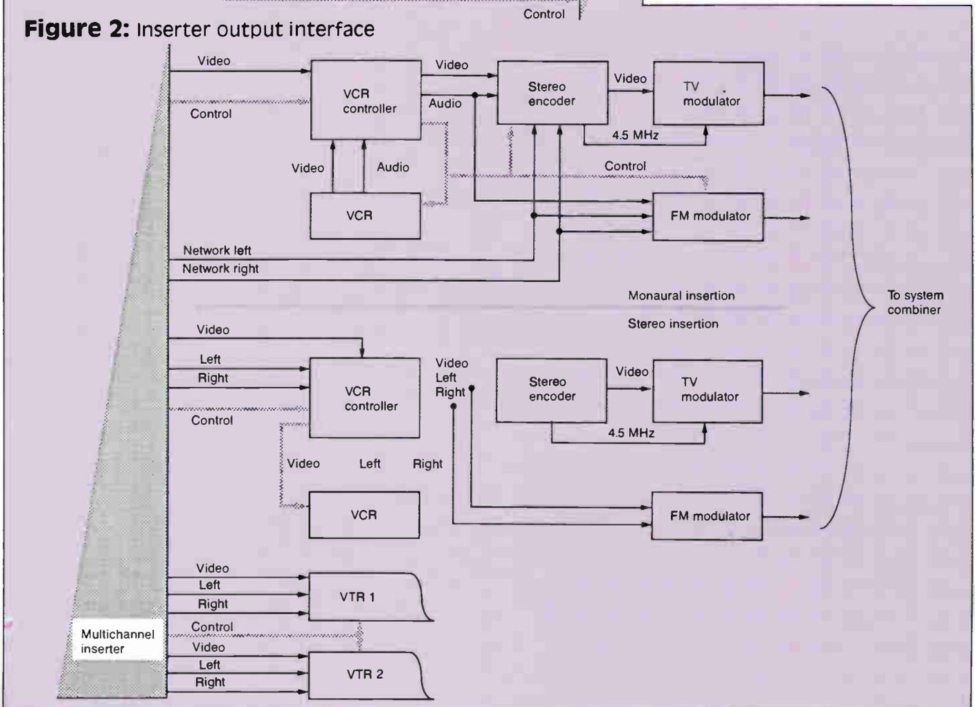
**"Promos may be inserted in mono or stereo, with selection on a channel by channel basis."**
