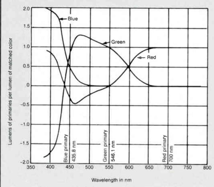
**Figure 3b:** Color mixture data of Figure 3a, replotted in terms of the power (watts) of the three standard real primaries required to match one watt of spectral color at various wavelengths as measured by a scanning spectroradiometer
