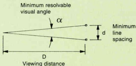
**Figure 2:** Resolution related to viewing distance and screen size
