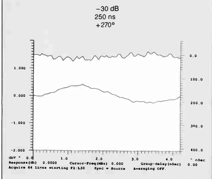
passive devices. The drop termination is generally considered a relatively poor match of only a few dB, and the potential exists, especially in cases with splitters feeding extra outlets, for reflections in the 100 ns range in excess of the threshold of perceptibility for either of the impairment functions.
