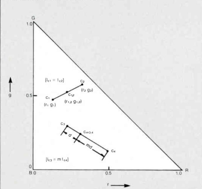
**Figure 6: Mixture of three colors on the RGB diagram and resolution of a given mixture color into its primary components**
