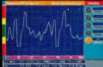
MLM display showing the video, color and sound carriers of Channel 3 with upper adjacent channel picture carrier and lower adjacent sound and color carrier also shown.
