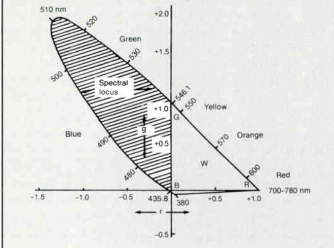
mixture color  $c_{1,2}$  is located at the center of the line joining  $c_1$  and  $c_2$ .
