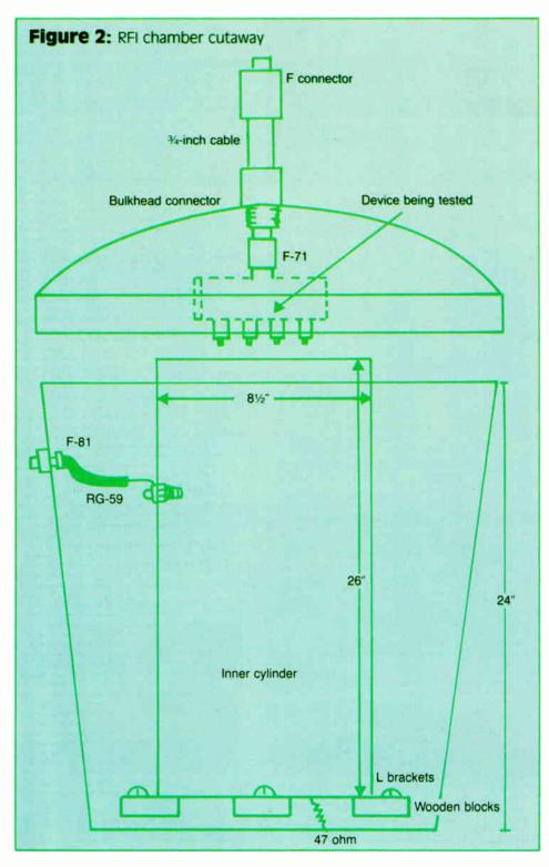
bolted to the cylinder. This F-81 is the point where the signal leakage is sampled. Because of the extremely low levels at the sampling point, the output is amplified by a post amplifier with 40 dB gain. Though only one frequency is inserted at a time, it is helpful to monitor and measure the amplified output with a spectrum analyzer like the HP Model 8559. This way you can vary the input frequency and still constantly monitor the signal leakage output
