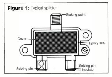
a small hole that only fits RG-59; some have a large hole for RG-59 and RG-6 and some have a tapered hole so that the center pin is guided directly into the seizing pin. This last type is preferable and will prevent a bent center conductor from bending further and shorting upon installation.
