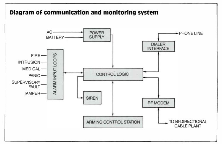
technology has evolved. Today, it is possible for home alarm terminals to monitor multiple zones for intrusion, smoke and heat or panic alarms (fire, medical or assault). Distinct condition-type alarms also can be transmitted to indicate signal loss, low battery and tamper.
