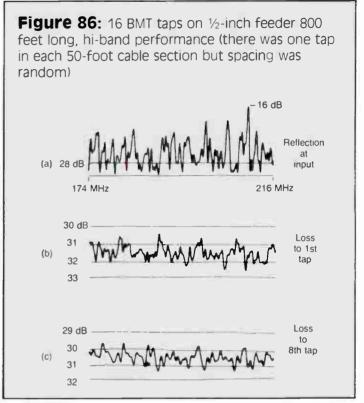
**Figure 87:** 16 CMT taps on  $\frac{1}{2}$ -inch feeder 800 feet long, high-band performance (there was one tap in each 50-foot interval but spacing was random)
