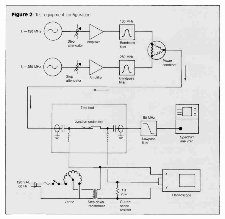
were searched for. None were found down to the noise floor of -80 dBm. This performance is adequate for the testing described in this article.
