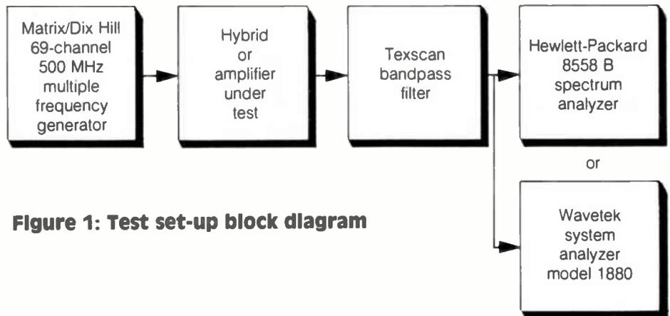
Figure 1: Test set-up block diagram
