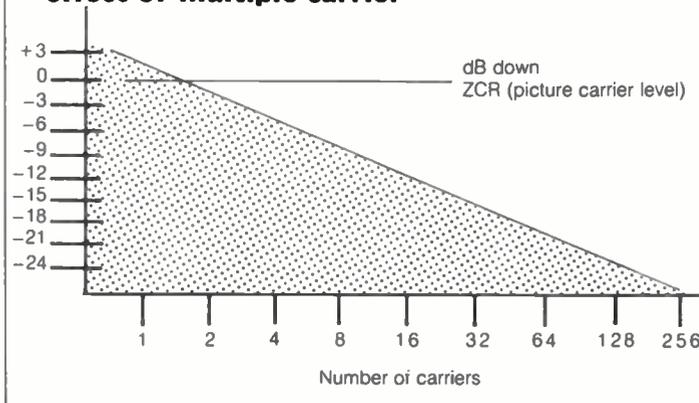
**Figure 3: Noise floor reduction with bandwidth reduction**
