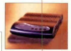
signaling protocols and an Internet protocol (IP) routing mode that supports routing information protocol (RIP) and network address translation for added security and network address preservation. The device is CableLabs-certified to DOCSIS 1.0 and is DOCSIS 1.1-ready. For more information, contact the company at (408) 526-4000, or visit www.cisco.com/go/cable.
