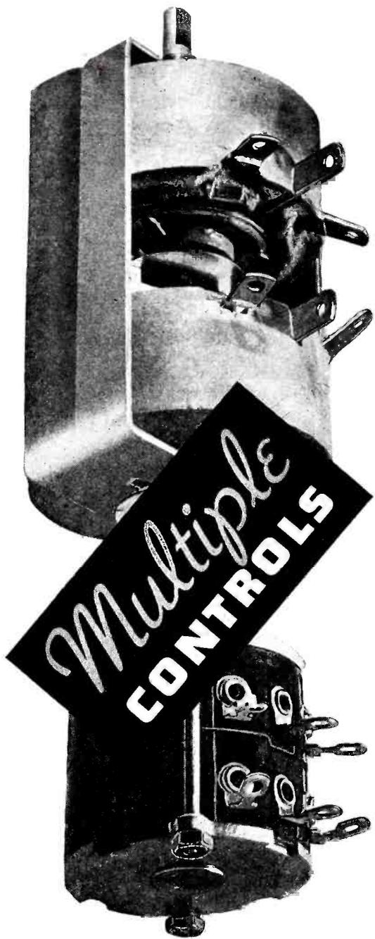
★ Another control problem—the kind Clarostat engineers like—came in recently. Specifically: a tandem assembly comprising dual 50-watt power rheostats and dual 3-watt wire-wound potentiometers; the latter insulated from shaft and ground for 2000-volt breakdown test; four units to have the same degree of rotation. In a hurry, of course; first a sample; then production running into large figures.
