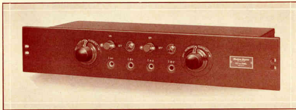
No. 217-A Panel for controlling the power to condenser microphone amplifiers, when this type of microphone is used.
